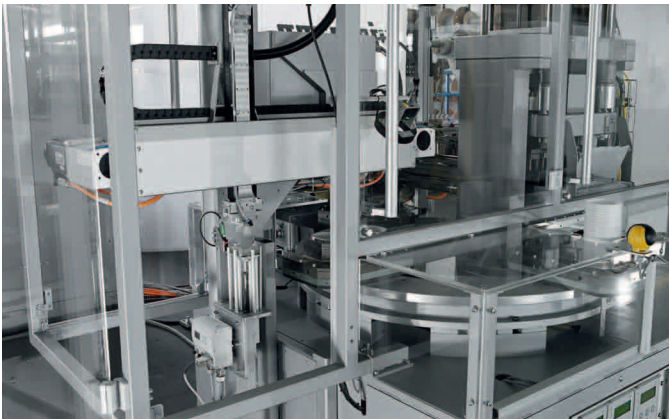
A glimpse into the secret life of an ultrasonic welding machine. Left: the high-speed T-gantry.
