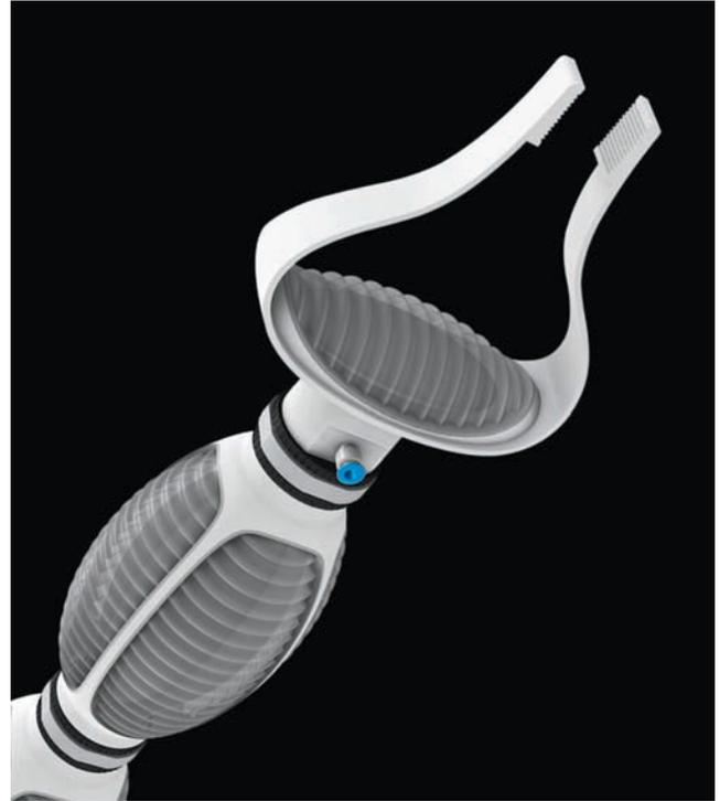
spatial and partly superimposed muscle configuration. The concept of generating multi-axis movement patterns by means of three-dimensional pneumatic structures, with no association of mechanical cause-and-effect relationships, became the new objective.
