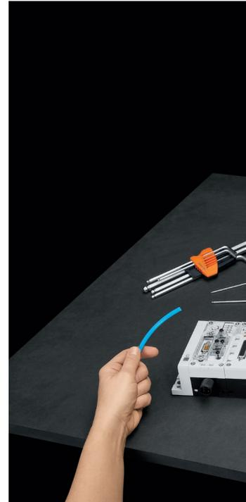
In order to keep the effort of tubing the BionicSoftHand as low as possible, the developers have specially designed a small, digitally controlled valve terminal, which is mounted directly on the hand. This means that the tubes for controlling the gripper fingers do not have to be pulled through the entire robot arm. Thus, the BionicSoftHand can be quickly and easily connected and operated with only one tube each for supply air and exhaust air.
