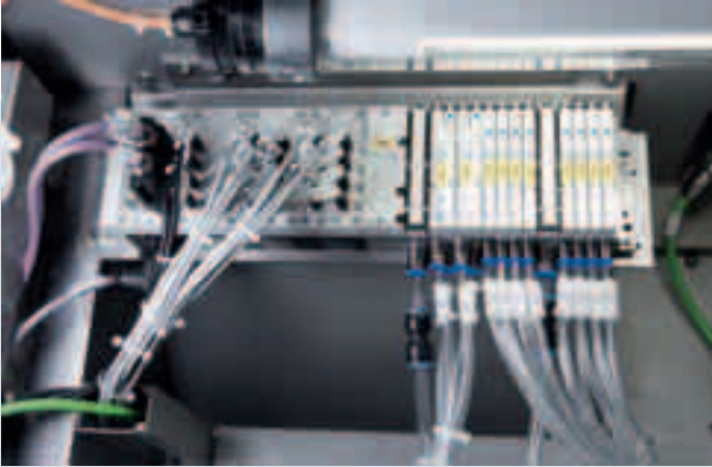
The valve terminal block MPA controls all the machine's pneumatic drives. The input modules of the CPX module process the sensor signals.
