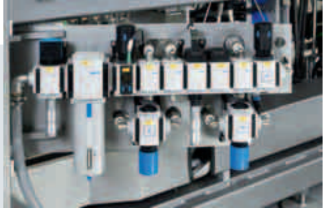
The MS-6 service unit including the safety soft-start/quick exhaust valve MS6-SV ensures that the OYSTAR IWK machine is provided with compressed air reliably and safely.
