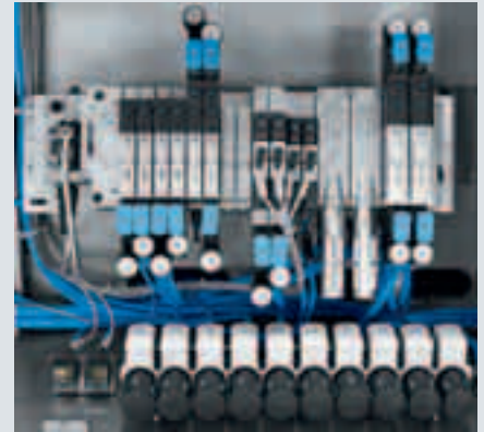
High flow rate is the decisive factor: the valve terminal VTSA's outstanding performance in the cartoner.
