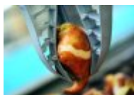
Caption: Adaptive gripping: a Festo proportional pneumatic valve VPPM ensures that the pressure exerted by the gripper fingers of the adaptive gripper DHDG is correct. (Photo: Festo)
