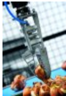
Caption: Sorting bulbs according to size and quality: the adaptive gripper DHDG is much more efficient than human hands. (Photo: Festo)
