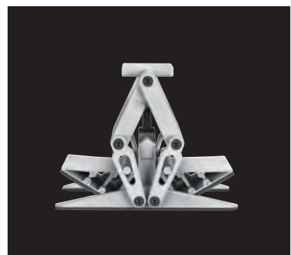
NanoForceGripper: energy-efficient gripping using the gecko as a model
