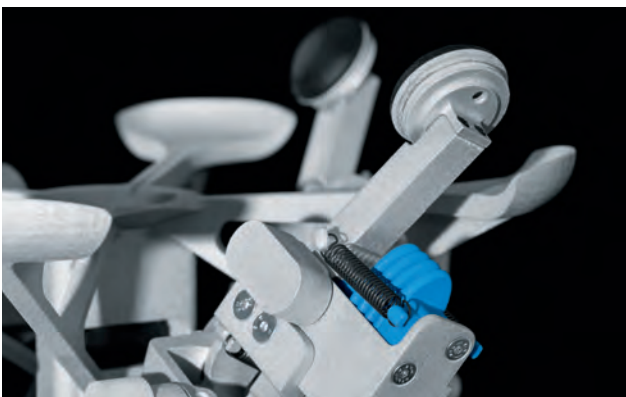
Self-learning: The LearningGripper's four pneumatic fingers ...
