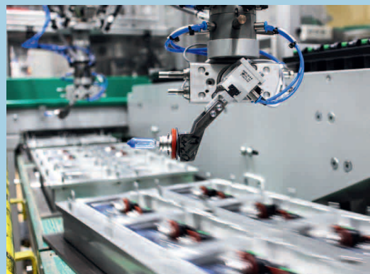
Highly dynamic: tripods type EXPT ensure a fast packaging process for car lights.
