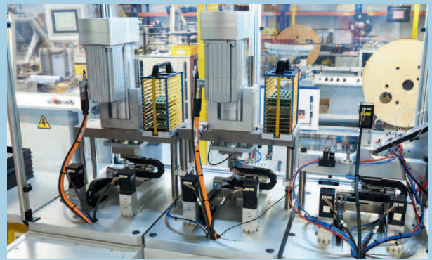
Modular design: the three stations of the Gecko assembly line for inserting, press-fitting and bending the contact pins – designed using standard components from Festo.
