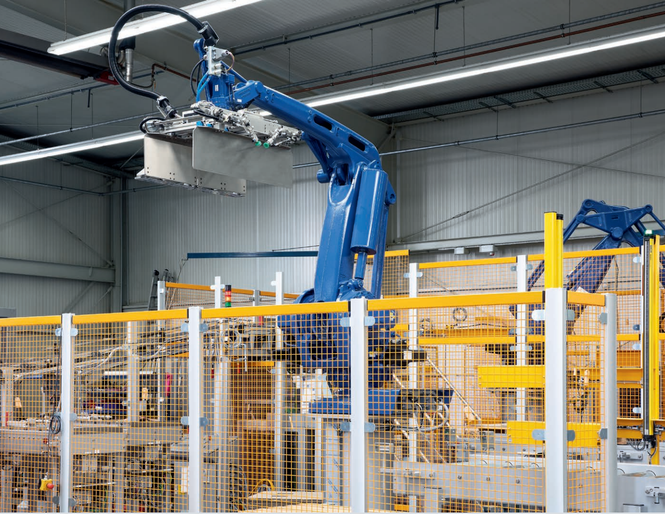
Optimal use of space: this palletising system forms the end of a highly automated packaging line.
