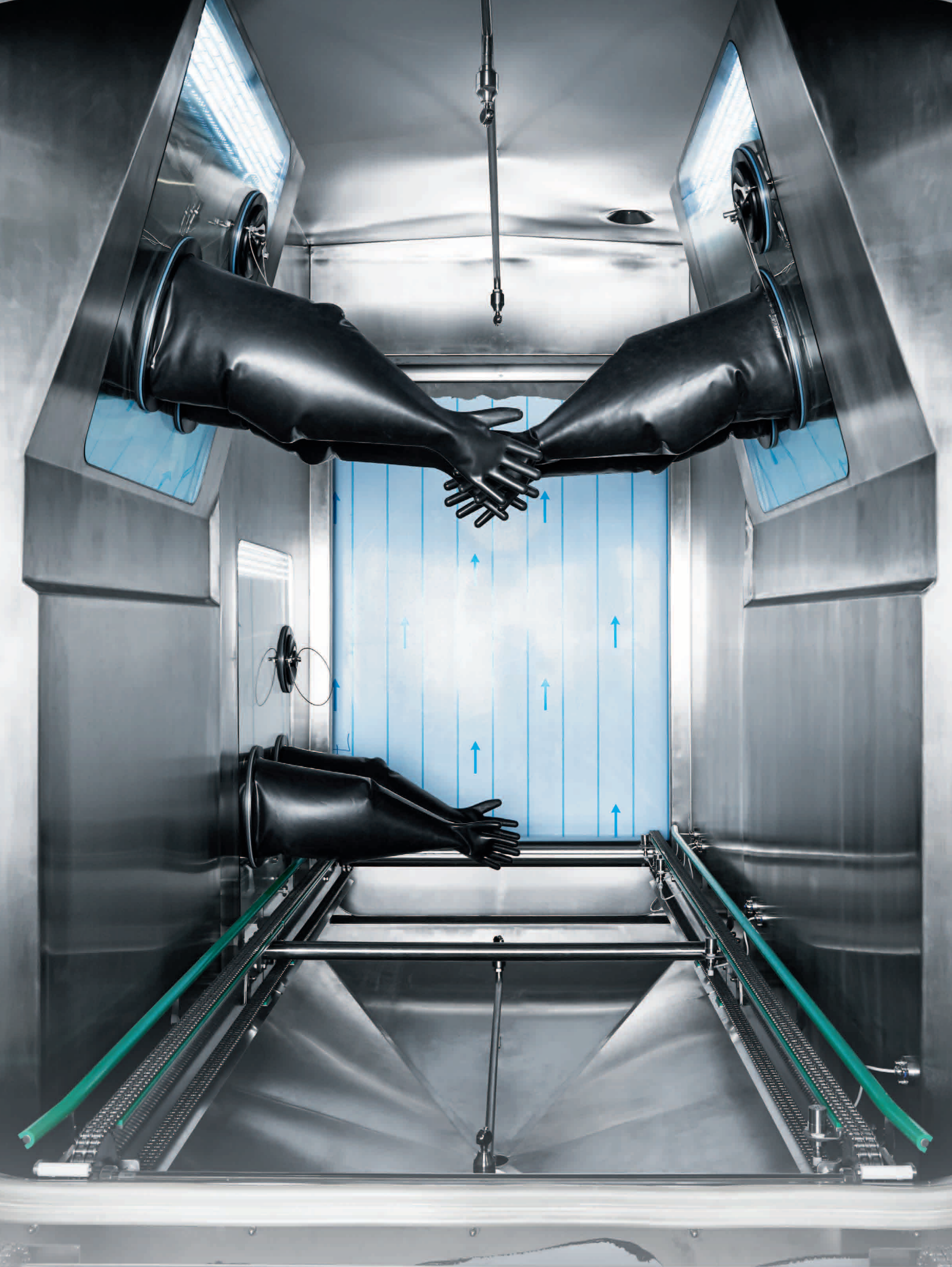
Reliable cleaning: safety cabin for opening the vessels using rubber gloves.
