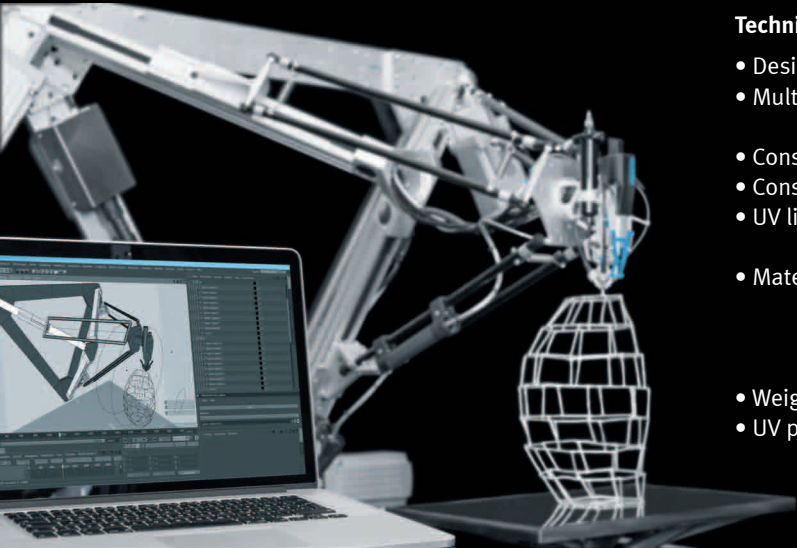
Digital production: the software transfers the geometry of the structure directly to the parallel kinematic system's motion paths.
