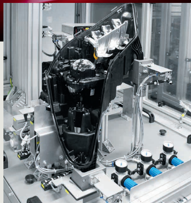
DSL swivel/linear drive units pull on the light module and check that it is firmly positioned.
