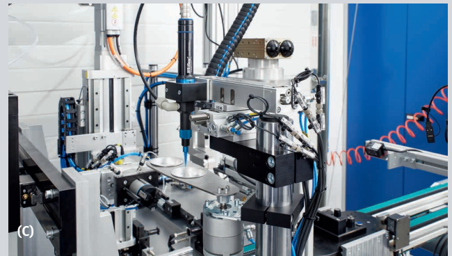
(A) The first of the three fully automated workstations rotates the workpiece carrier 180 degrees using a cylinder DRSL and fixes it in place using a holding unit controlled by a mini slide DGSL. (B) Twin-piston semi-rotary drive DRRD with three-point gripper DHDS for picking up the workpiece for machining. (C) A semi-rotary drive DRVS moves two drip trays below the dosing nozzle, thus protecting the system against contamination.
