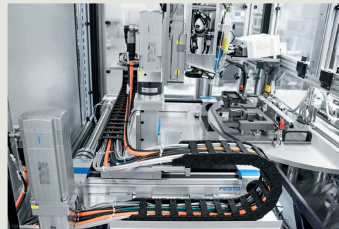
A ready-to-install handling system ensures even application of a two-component thermally conductive paste.
