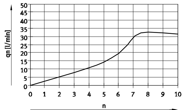
Standard flow rate q_n at 6 → 0 bar as a function of turns of the adjusting screw n
