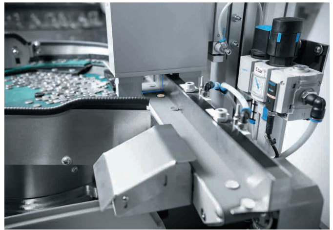
The checkbox CHB-C-N checks the metal discs and controls the entire sorting process. The position and quality inspection is carried out completely contact-free
