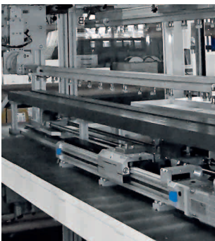
An electric linear gantry positions the strings as gently as possible to prevent cell breakage
