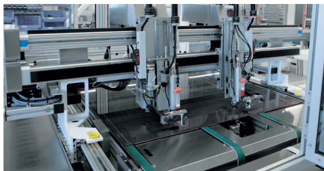
Two dispensing heads that work in parallel and can be positioned independently of each other apply the adhesive beads to the thin-film cell
