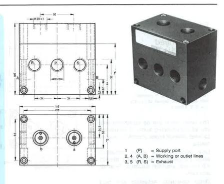
In its centre position, this valve holds the piston of a double-acting cylinder clamped under pressure.
