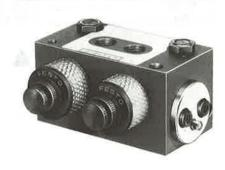
The valve can be reversed as desired, either manually by means of the switch lever, mechanically via switching stems by actuating the built-in 3/2-way valves, or pneumatically by means of a signal to port Y or Z. The speed of the advance and return strokes of a cylinder is controlled by exhaust port flow control and can be set on the two regulator screws.
