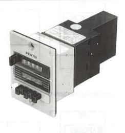
Times are pre-selected by pressing the white locking button and simultaneously keying-in the pre-selected value. The pre-selected time setting is retained when the timer is reset.
