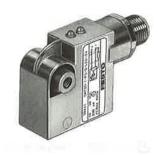
These proximity sensors are used in welding installations with strong alternating magnetic fields for contactless position indication with Festo cylinders series "A", piston dia. of 32 to 100 mm with tie rod.
