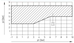
① Operating range for valves with external pilot air supply
