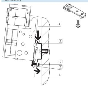
The CPA-SC valve terminal is attached to the H-rail (see arrow A).
