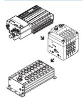
The optional string extension allows additional valve terminals and I/O modules to be connected to the field-bus node of the CPA-SC. A CP string of the CPI installation system is integrated in the fieldbus node as an extension. Different input and output modules as well as CPV- and CPA valve terminals can be connected.
