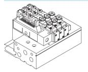
With this electrical connection variant, all valves are centrally actuated via the 26-pin connector
