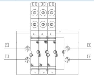
The CPA-SC valve terminal is screwed onto the mounting surface using four M4 screws.
