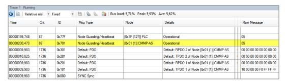
• You can switch off the Heartbeat mechanism when you set the node heartbeat producer time to 0.
