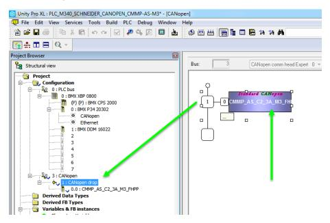
•Please set the number of PDO's for 'receive' and 'transmit'. Depending on your settings in FCT (FCT...Festo Configuration Tool) you need different numbers of PDO's (FHPP, FHPP and FPC, FHPP and FPC and FHPP+). In the following example we are using FHPP and FPC, which means 16 Byte IO resulting into two TxPDO and two RxPDO.
