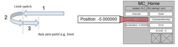
To set the axis zero point according sequence 3 a **negative** position value (-5.0) is required. That means to move the sequence 3 in the opposite direction the position value has to be **positive** (+5.0).
