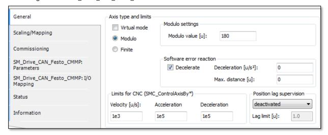
And in Scaling/Mapping configuration the scaling is done accordingly to the used gearboxes and the wished user unit in degrees:
