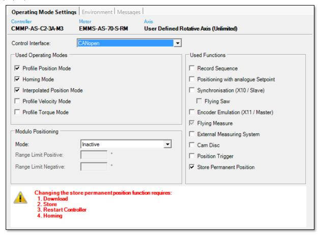
Do not select the modulo function on the motor controller side, i.e. keep "Modulo Positing" to Inactive. The activation of modulo calculations in the motor controller will change the position values sent to the PLC and leads to problems within Softmotion. For Softmotion we always should sent the unchanged position value via the fieldbus interface.
