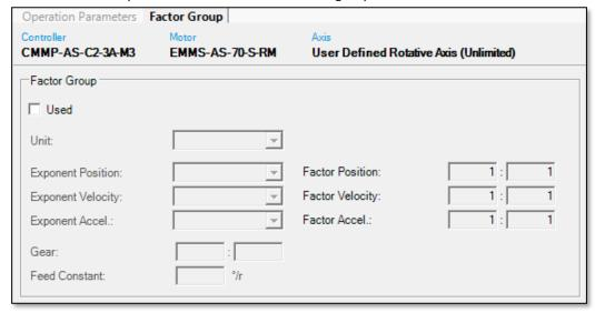
Not using the factor group means that the units of position values which are exchanged via the fieldbus are related to the motor shaft (1 rev =  $2^16$  inc) and all the scaling to user units will be done solely on the Softmotion side.
