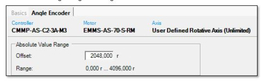
The first overflow of the multiturn encoder happens at 437 feed movements as then the actual position first time exceed the upper limit of the 12 bit multiturn counter.
