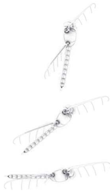
Fig. 7 Different positions in space while hovering. With dragonfly-inspired MAVs it becomes possible to take different orientations in space while flying or hovering by twisting the four wings in regards to the body plane. Here the different wing positions during hovering are shown, when BionicOpter hovers in the vertical (upper picture) or horizontal (lower picture) plane. An intermediate state is shown as well.
