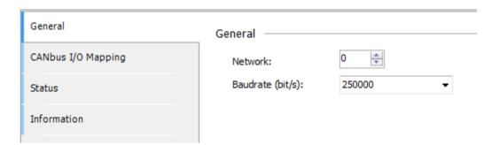
**Network** refers to the assigned CAN interface being used. If only one interface is available, network number must be 0. There are no current Festo Devices within CODESYS V3 that have 2 CAN cards, so it should always be set to 0.
