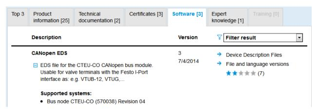
To install open CODESYS V3 and go to Tools -> Device Repository.
