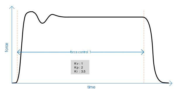
A force control function can be used with precontrol only and a very short holding time, in order to reduce overshooting. Kp and Ki are activated as required by means of the second force control function.
