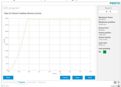
Force-time diagram where Kv = 0.8, Kp = 2 and Ki = 5, roughly 402 N is reached:
