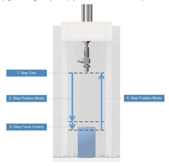
The force sensor is tared to an initial value at the initial position. That is positioned in front of the component and is pressed using force control. When the pressing operation has been completed, retraction to the initial position takes place.
