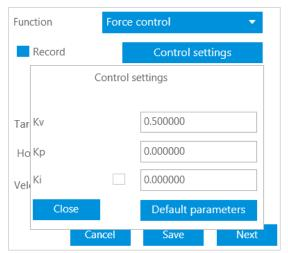
• All parameters have been set. A reference curve is then recorded in "Step 2/4: record/loading reference curve". If target force is not reached, waiting is required until the time limit has elapsed, or the process can be stopped manually. The force-time diagram is reviewed for the purpose of analysis:
