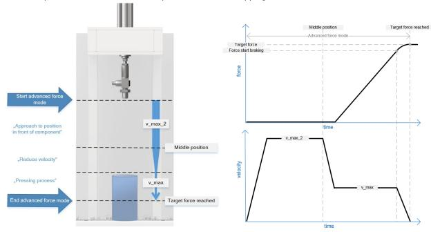
With this switching of the speed, the cycle time can be reduced in contrast with a separate positioning step. This is illustrated in the following diagrams:
