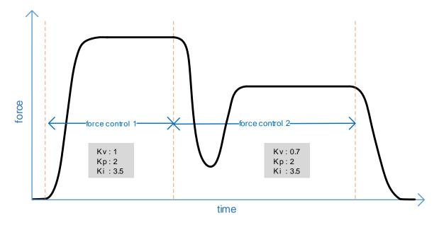
An additional force control function must be included in order to reduce this decrease in force. This function makes use of precontrol only, and thus prevents excessive decreases in force. Force control function parameters have to be adapted individually in this case.
