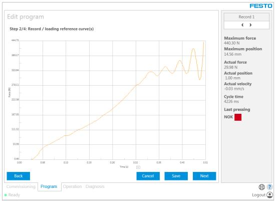
→ The controller is rendered instable and starts to oscillate due to the excessively high Kp value. The "maximum force" limit value stops the process.
