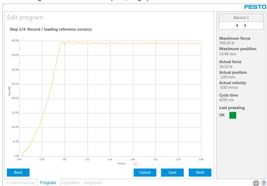
• Force-time diagram where Kv = 0.8 and Kp = 1, roughly 399 N is reached:
