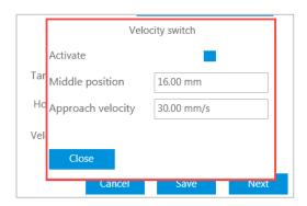
**Note:** The velocity is not reduced until the middle position is reached.
