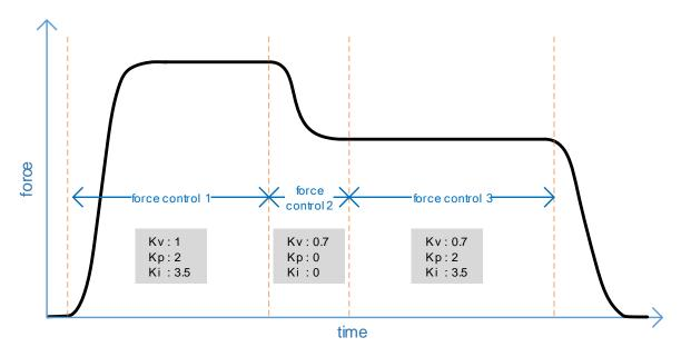
**Note:** Selected maximum speed is only complied with in the case of positive force build-up. In contrast, maximum speed is complied with even when force is reduced in the case of advanced force mode.
