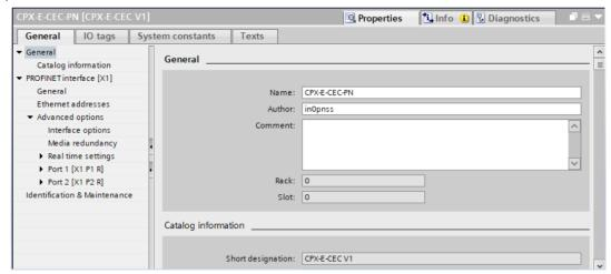
4. The network parameters are under Ethernet Addresses.
