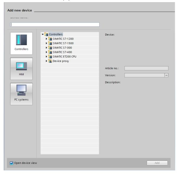
5. If the PLC and you PC are connected in the same network, then it will be easy to do the PLC configuration if we can retrieve the actual hardware configurations present at the PLC. So for this purpose select **Unspecified CPU 1200** from the list of available CPU's as shown below.
