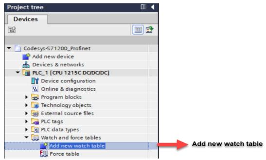
2. Map the Input addresses of the Profinet Module to the watch table.
