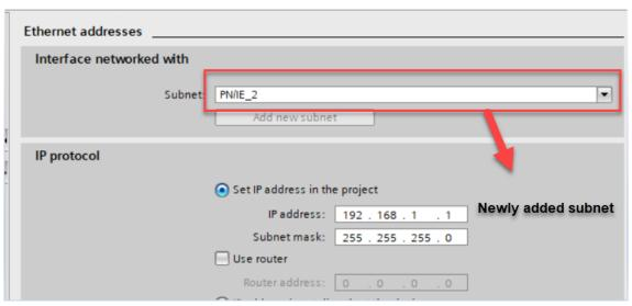
4. Enter the needed IP address and subnet mask in the IP protocol part of the ethernet addresses.
