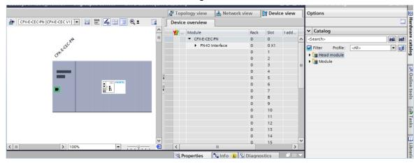
3. From the catalog select the needed Profinet IO module.
