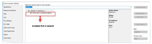
7. Double click on the available PLC to set the path active. Once the path is active the selected PLC will be bolded as shown below.
