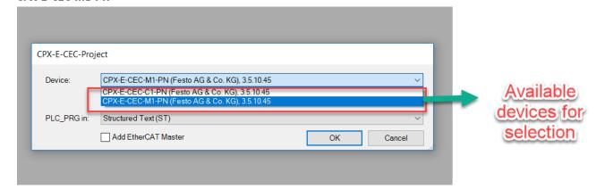
We will use CPX-E-CEC-C1-PN as we have to establish Profinet communication with S71200/1500 PLC.
