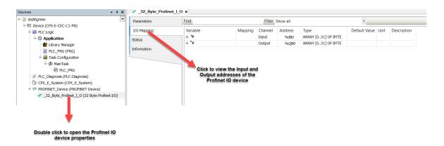
6. The profinet IO variables updation setting will be by default "Use parent device setting".
