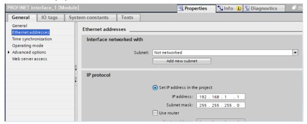
3. In the Ethernet Addresses properties click on Add new subnet to create a new subnet as shown below.
