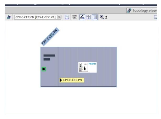
2. **Click on CPX-E-CEC-PN module** to view the properties of the controller.
