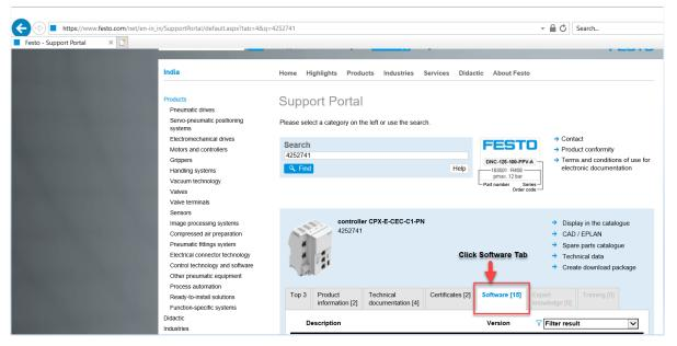
3. Under Software category scroll down until you find the Profinet GSDML File for CPX-E-CEC controller.
