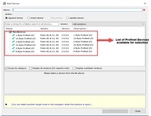
3. Click On the needed Profinet Device and Click on **Add Device**. In this example we are considering selection of **32 Byte Profinet I/O**.
