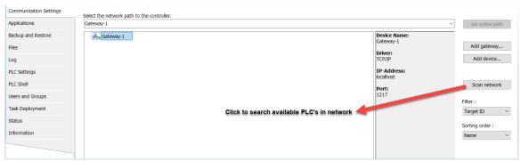
6. If the PLC is connected to the network the PLC will be listed in the gateway as shown below.
