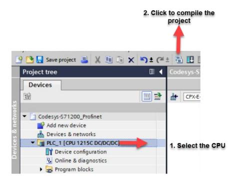
2. Once the compilation is finished with no errors, then the project can be downloaded to the PLC.
