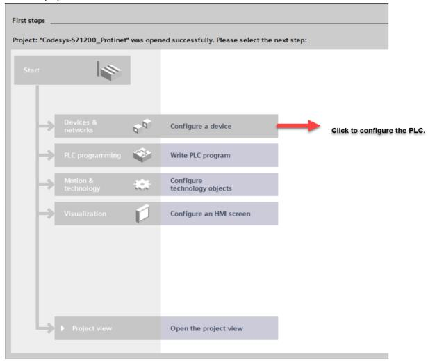
4. Click on **Configure a device** to do the PLC configuration as shown in the above image. The configuration screen allows you to choose the PLC CPU needed from the available list of CPU's.
