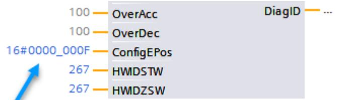
Since bit 0 and bit 1 are already set, input variable "**ConfigEPos**" must be set to **16#0000\_000F**.
