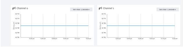
In addition to the parameters summarised in the widget area, historical data is available for CSV export. The data is read out without unit of measure. The measured values displayed here are raw values and correspond to those of the unit of measure selected in the module. If the selected unit of measure is known in the hardware, the data can be interpreted clearly.
