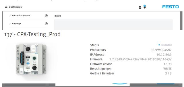
Note: If a gateway cannot be deleted, first determine whether or not the gateway is set to switch position 3 = Read/Write. This can be checked on the Gateway page. "WRITE" authority must be available here. If there is no
