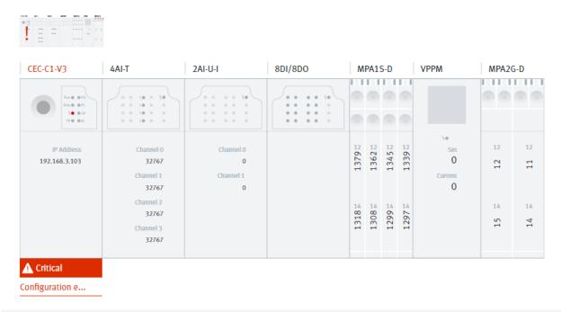
A thumbnail view can be seen above the illustration. This displays the area of the valve terminal in which you are currently located. This is necessary if large CPX configurations are available and the display range is insufficient. This thumbnail view can also be used to move the displayed area. A red exclamation mark also identifies the module at which an error has occurred (e.g. critical limit violation, parameterisation error etc.).
