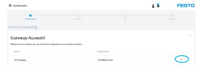
Here, you can now choose between two scanning procedures. During auto-scan, the gateway scans the field level and then lists all devices that can be boarded. By scanning manually, you can search for a specific device when the IP addresses are known. Basically, no distinction is made between the boarding statuses of the two scanning methods. The devices which are compatible with the dashboards are listed.
