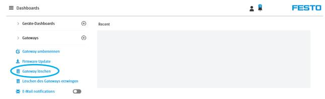
The "Delete gateway" window then appears and you are prompted to set the switch at the gateway to position 3 = Read/Write. When this is done, close the window by clicking on the "Cancel" button.
