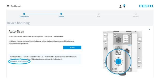
If manual scanning has been selected, an IP address must be entered in step 2, "Scan Mode". Once this has been done, you can click on "Next". Now the gateway searches for the network participant with the entered IP address.
