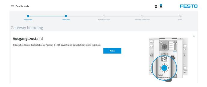
In the next step of the boarding process, turn the switch at the gateway clockwise to position 1 = Onboarding. A connection is now established between the gateway and the cloud. As soon as the connection has been established, the "Next" button is enabled Click on "Next".
