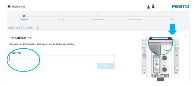
Then you can continue with the next step of boarding. Set the switch at the gateway to 0 = Off, after which the "Next" button is enabled. Now click on "Next".
