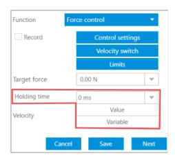
• *Velocity:* The maximum possible velocity during the pressing procedure (v\_max).
