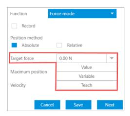
Maximum position/Maximum distance: if this value is exceeded before reaching the target force,
