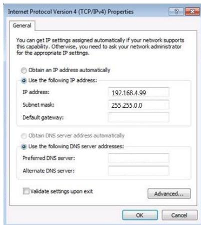
You can set the IPs (CECC-X and CMMP) with the Festo Field Device Tool (FFT). Open FFT and scan your network. You should find minimum the CECC-X and CMMP.
