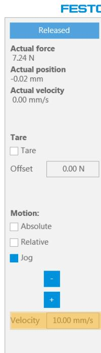
With the buttons “+/-“ you can now move the cylinder in positive and negative direction.
