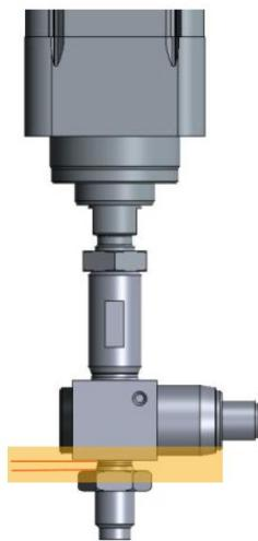
Connect the cable NEBU to the sensor.
