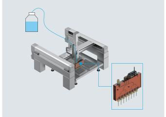
The process is based on just a few parameters: you define how much liquid is dispensed into the wells of the microwell plates as a function of the pressure in the reservoir, the needle cross section and the valve opening time.
