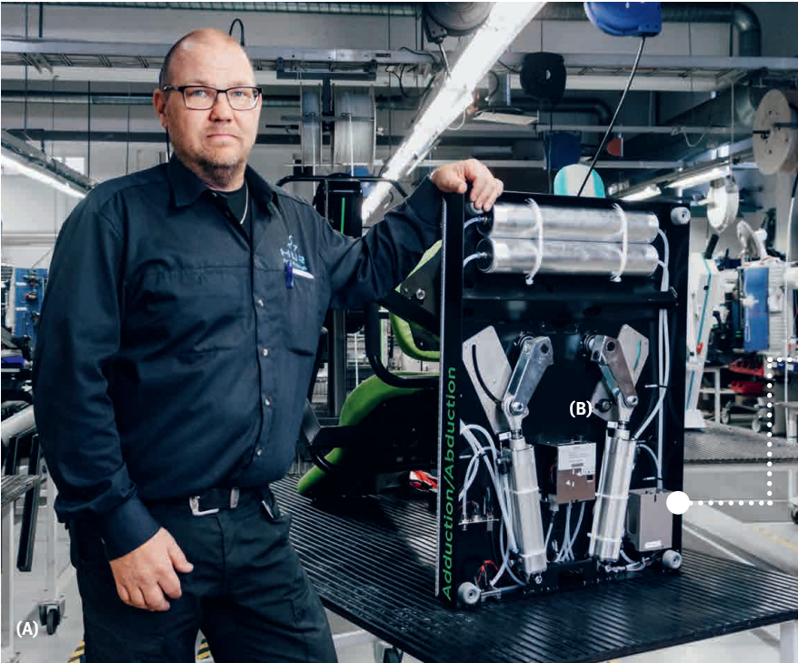
(A) Pneumatic fitness: no inertia effect in training equipment with the standards-based cylinder DSBC and the pre-assembly for controlling the actuators. (pictured: Markus Högnäs, Plant Manager at HUR).
