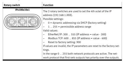
From Festo manual p/n 8099750, set switches to 608, 600 being the least significant value for Modbus
