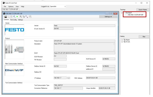
3. Go to the Port Config tab. The Port addresses of the IOL master will be represented by the module number, and port number of the module. Press the Green Arrow to go on-line.
