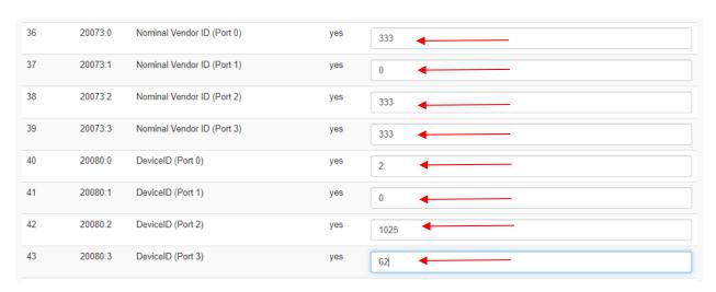
7. Export this configuration to the controller using Stored Parameters to save this configuration in the CPX-AP Ethernet adapter. Connect the controller and RUN.
