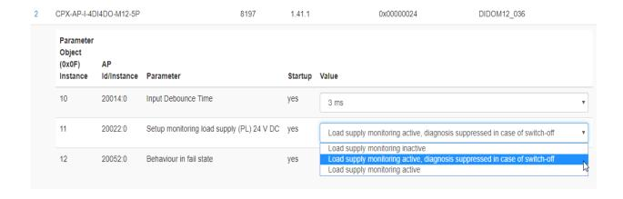
Some modules, such as the 4 channel analog input may have an extensive list of parameters. The 4AI module has 52 parameters for configuring the 4 analog channels. Some parameters are required, such as the signal range, so it matches the sensor connected.
