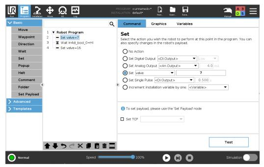
• In this case, a value of 7 is set to the name "valve", which was assigned to the first Output Register of the VAEM module of the VTUG valve manifold. This is address 1 in this example. When this sequence is executed, the value 7 (0000 0000 0000 0111) is set, and the first 3 coils are energized.
