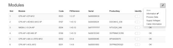
The Process Data focus shows the actual I/O status, dynamically, with an update rate of about 1 second.
