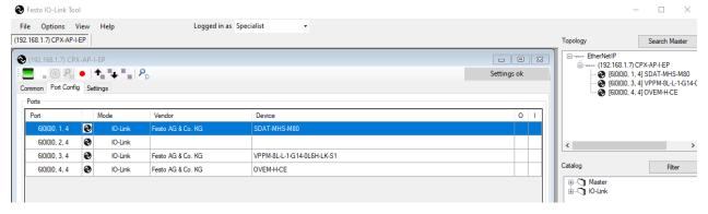
5. Double click on a device to open its IODD parameters and other information available from the IODD file. Follow the manufacturer's instructions from each device on setting parameters or other actions. In this example, the SDAT Position Transmitter is opened.
