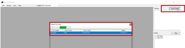
2. When complete, double click on EtherNet/IP master. The master page will appear. The master will be shown in the Topoloogy Window.
