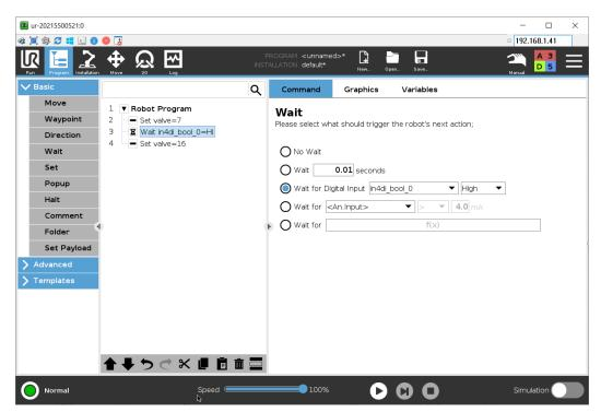
In this case, a delay is added. A new value of 16 (0000 0000 0001 0000) is set. The 5<sup>th</sup> coil only is now energized.
