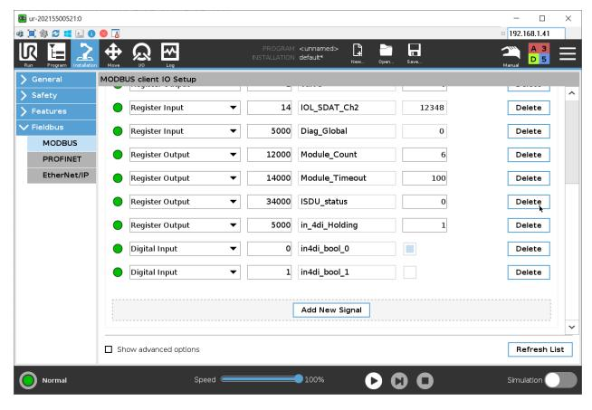
You can also use Digital Input and Digital Output to set coils and read limit switches individually
