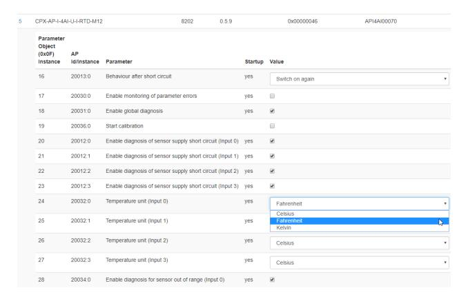
The IO-Link module also requires parameterization. By default, all the channels are deactivated. When using the IO-Link master(s), certain parameters need to be configured. Primarily:
