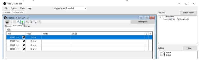
4. Once on-line, a Green Bar will indicate on-line is active. Click on "Check Devices", and a window will appear showing the connected devices at each port. Select "Takeover devices into engineering".
