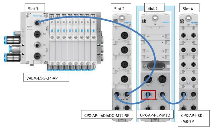
The right AP-I connector is the Secondary branch of the AP-I system. Modules connected to the Secondary branch start consuming slot numbers after the last slot number of the Primary branch. The above example shows the completed test system with all 4 slots consumed.
