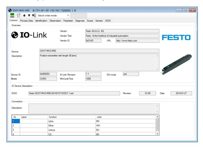
Go to the parameter TAB, and change the BDC1 Switchpoint mode from deactivated to Window comparator. Note the yellow "c" for changed, edited vs. "i" for initial.
