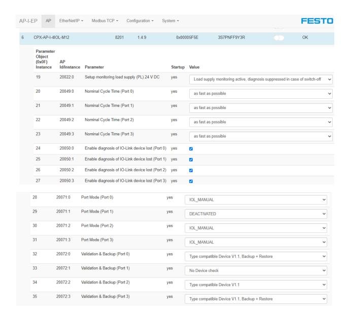
8. Go back to the IO-Link SW Tool to check. Going back on-line will now show the port configuration from the data stored in the CPX-AP from the Stored Parameters.
