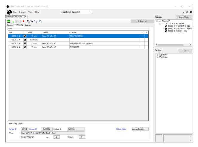
9. Double click on the SDAT device in this example in port 1. Go to the parameter tab and then select the up-arrow for "upload from device". The state of each parameter is synchronized with the device and the window comparator setting is still loaded in the device.
