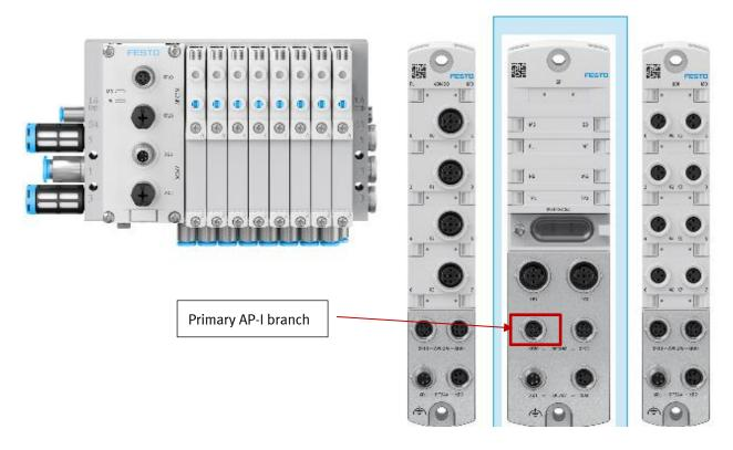
The CPX-AP-I-EP adapter is always slot 1 of the AP system. The left AP-I connector is the primary branch. All modules connected to the primary branch consume the next available slot numbers, in order of connection. The leftmost AP-I connector is the incoming branch (topmost for pneumatic), the rightmost is the outgoing branch.
