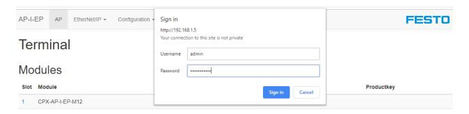
Each module can be configured by clicking on it. For example, slot 1 is the Modbus adapter. One click on the module opens the parameter selection list for the module.
