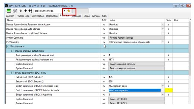
Select the yellow down button for "write all changed values to device". The yellow "c" changes to a green "d" indicating the tool is synchronized with the device. Go off-line from the IO-Link Tool.
