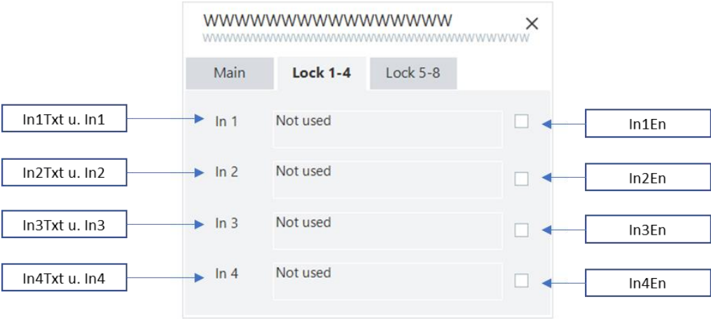
Fig. 117 LockView8 Lock1-4 Faceplate
