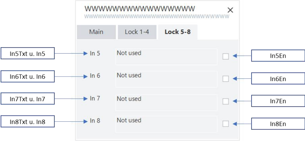
Fig. 118 LockView8 Lock5-8 Faceplate
