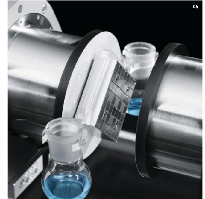
In the future, many manufactured products will move quietly and cleanly through the production shops, with low energy consumption and without contact. The hovering transfer of objects beyond system limits not only makes longer process chains without contact possible, but it also enables low-maintenance use in surroundings with strict cleanliness requirements.
