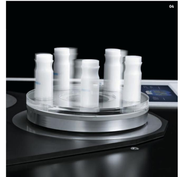
Superconducting automation modules can be implemented with a number of active drives. That enables them to perform even unusual motion sequences, positioning forms and handling processes whilst hovering.
