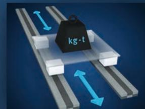
**SupraLinearMotion:** frictionless, linear gliding using gravity
