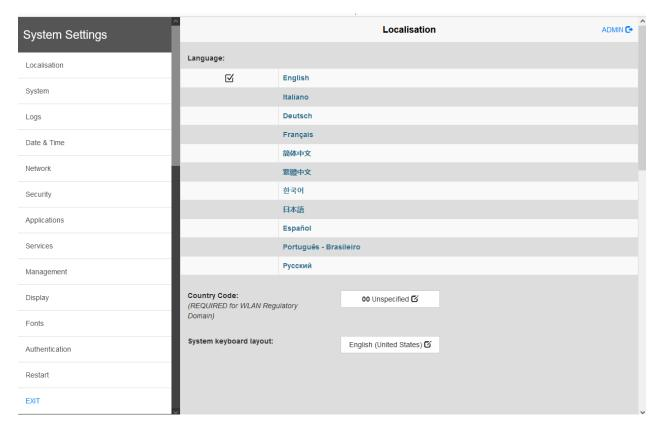
The active item of menu is highlighted on the left side of the screen. The right side shows related information and settings. Depending on the size of the HMI screen, both menu and content of selected item may be shown on screen at the same time or not.
