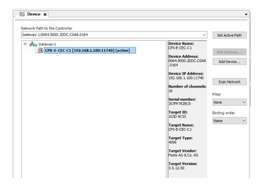
• Then CODESYS programs can be loaded onto the controller (without gateway service) as usual. The burst-like broadcasts caused by the gateway service are thus eliminated and no longer lead to a connection abort between the VAEM-V and the controller.
