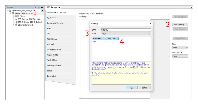
• Select TCP/IP under "Driver" and enter the IP address of the controller for the gateway. The controller and the PC must be in an IP network (e.g. with subnet mask 255:255:255:0 | PC 192.168.1.99 | SPS 192.168.1.100).
