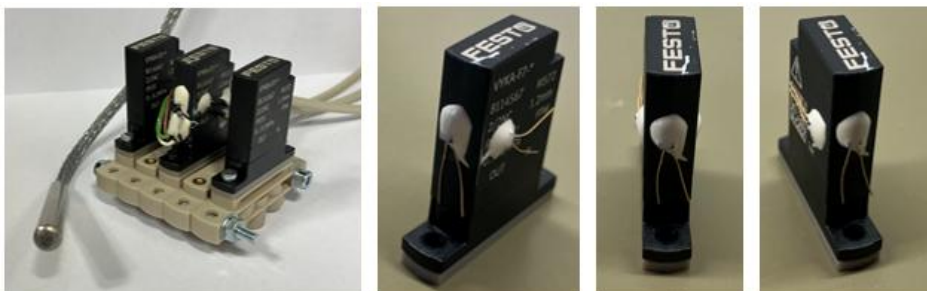
Figure 6: Temperature sensors on VYKA valve
