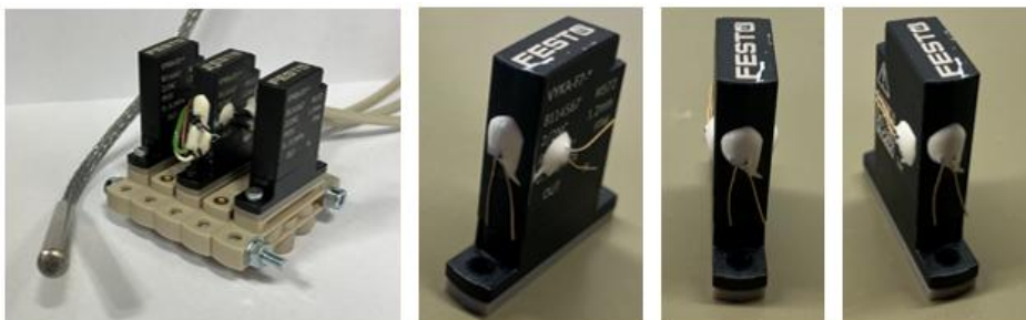
Figure 6: Temperature sensors on VYKA valve
