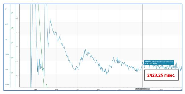
Calculation of the natural frequency:  $\left(\frac{1}{\left(\frac{Timemax - Timemin}{Numberpeaks}\right)}\right) * 1000$
