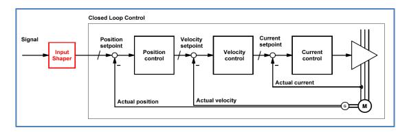
In order to achieve the desired results, the natural frequency of the system must be communicated to the **Input Shaper**.
