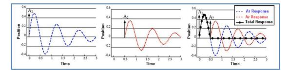
**Attention**: modifying the control signal results in a longer positioning time!
