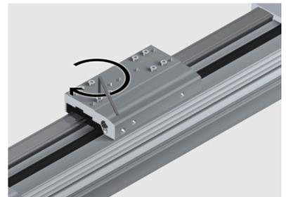
23. Clean the socket head screw to remove the threadlocker.
