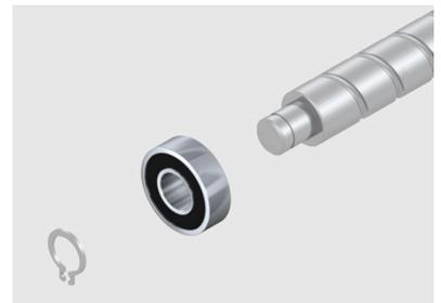
12. Apply a thin layer of grease to the inner raceway of the roller bearing.
