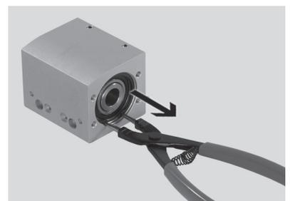
3. Push the toothed belt pulley module with the two deep-groove ball bearings out of the actuator end cap.
