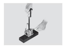
Unscrew the two free push-in fittings QS, Quick Star on the lower valve manifold.
