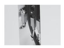
Remove the two pilot air tubes from the push-in fittings QS, Quick Star on the lower valve manifold.
