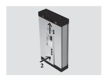
• Tighten the rear cover with the screw. The maximum tightening torque is 1 Nm.
