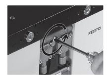
Remove the air nozzle from the valve manifold using a pliers.
