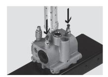
• Screw the two push-in fittings QS, Quick Star onto the lower valve manifold. The maximum tightening torque is 10 Nm.
