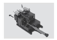
• The second solenoid valve is removed in the same way as the first.
