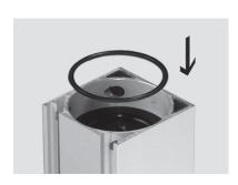
• Insert the upper metal cover with the new plastic disc (included in service kit) and the screw in the profile.
