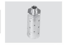
• Insert the new or cleaned silencer in the lower valve manifold and tighten it. The maximum tightening torque is 5 ±1 Nm.
