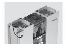
• Disconnect the tube with the upper valve manifold from the push-in fitting QS, Quick Star. Use an open-jawed spanner (SW 15) to push in the push-in fitting QS, Quick Star coupling and remove the upper valve manifold.
