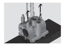
• Unscrew the silencer from the lower valve manifold.
