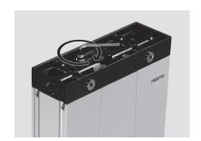
Tighten all four spacer bolts of the profile. The maximum tightening torque is 20 Nm.
