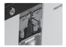
• Reinsert the mounting screw of the air nozzle in the upper valve manifold and tighten it. The maximum tightening torque is 3 Nm.
