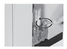
Unscrew the silencer from the lower valve manifold.
