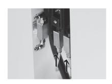
Insert the pilot air tubes into the push-in fittings QS, Quick Star on the lower valve manifold.
