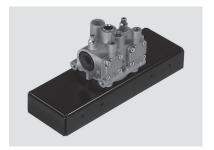
• Screw the lower valve manifold onto the base plate from underneath using four screws and washers. The maximum tightening torque is 20 Nm.
