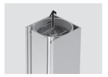
• Unscrew the screw from the lower gasket completely.
