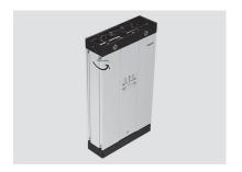
• Loosen each of the four screws in the distributor housing with three full rotations.
