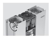
• Insert the two pilot air tubes in the push-in fittings QS, Quick Star on the lower valve manifold.
