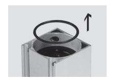
• Remove the ring fitting from the profile.
