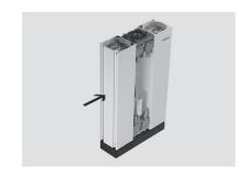
• Screw on the four spacer bolts of the left profile and tighten them. The maximum tightening torque is 20 Nm.
