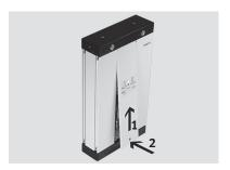
• Tighten the front cover with the screw. The maximum tightening torque is 1 Nm.
