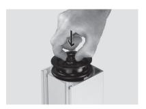
• Place a new large O-ring (included in service kit) on the ring fitting.
