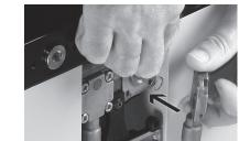
• Centre the housing cover on the tapered spring; the spring must sit in the circular indent in the housing cover.
