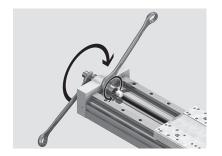
• Install the new shock absorber subassembly once again in reverse order and tighten the lock nuts with the appropriate tightening torque.
