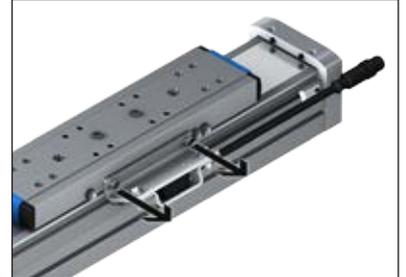
2. Unscrew the countersunk screws of the caps from the slot nuts at both ends of the magnetic strip.
