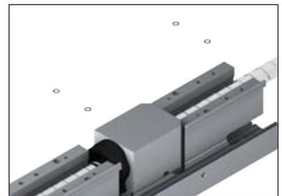
6. Wet the threaded holes for mounting the lubricating heads in the slide module with screw locking agent.
