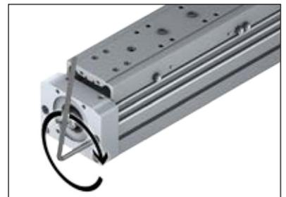
16. Push the slide module in the direction of the bearing cap until it stops.
