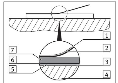
3. Adjust the magnetic strip (incl. steel strip) [1] with the adhesive strip side in the middle on the cylinder barrel. A distance of 20 mm each must be maintained from the bearing block and bearing cap.
