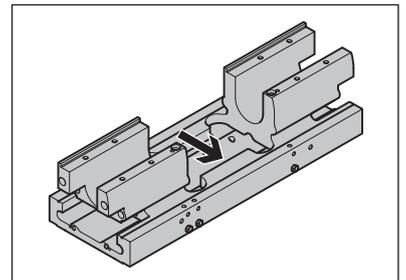
6. Press the entire contact area of the retainer or retainer assembly onto the stop edge of the slide module.
