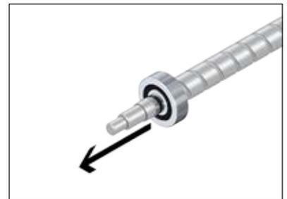
3. Apply a thin film of grease to the inner raceway of the new roller bearing.
