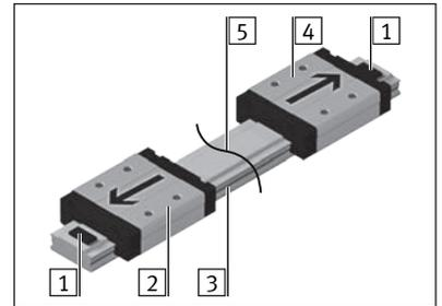
4. Place the slide module on the work surface with the attachment side facing downwards, the lubrication nipples face the **rear**.
