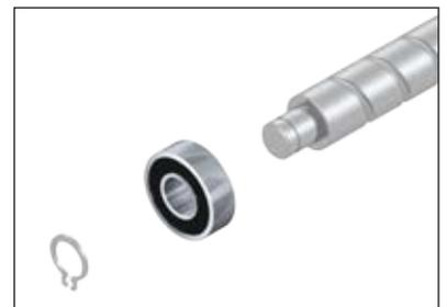
5. Apply a thin film of grease on the roller bearing with seat in the bearing block on the inner raceway.
