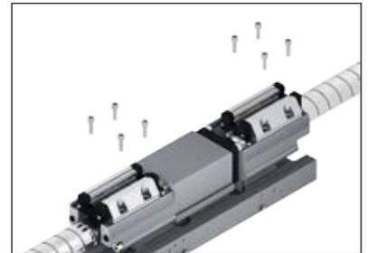
3. Unscrew the flange screws in the two barbed L-fittings of the lubrication.
