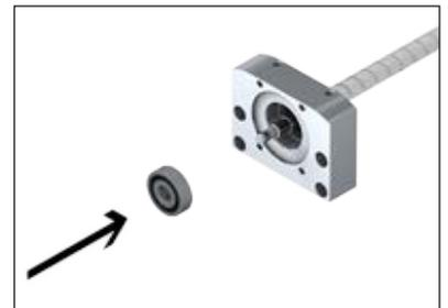
6. Apply a thin layer of grease on the outer and inner raceway of the roller bearing.
