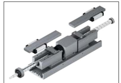
16. Carefully turn over the slide module with spindle assembly and the roller carriages and place on the assembly tools; the lubrication nipples face the front.
