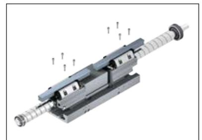
16. Push the roller carriage with the ground side onto the stop edge of the slide module and at the same time, tighten the socket head screws with the appropriate tightening torque.
