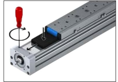
13. Place the clamping element on the cover band.
