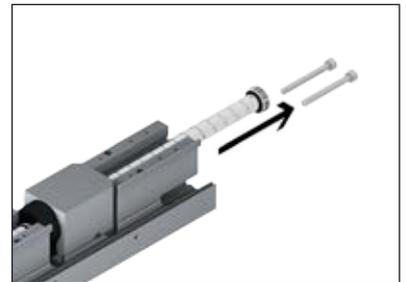
12. Remove the spindle assembly with retainer or retainer module from the slide module.
