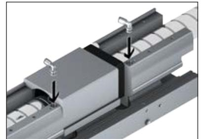
11. Screw in the flange screws and tighten with the appropriate tightening torque.
