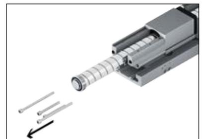
9. Remove the spindle assembly with the retainer module from the slide module.
