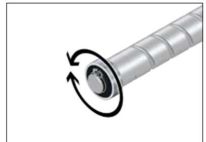
**Replacing the deep-groove ball bearing**
