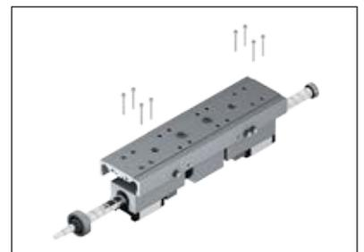
3. Turn the slide module with the mounted on spindle assembly through 180°. The roller carriages face upwards.
