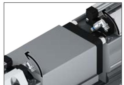
5. Remove the roller carriage from the slide module.
