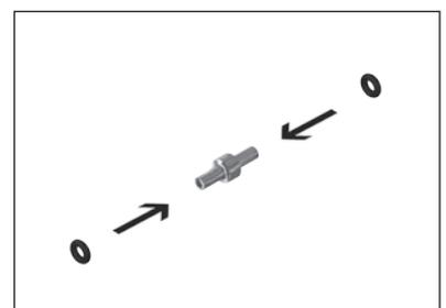
12. Insert the lubricating channels into the lubrication holes of the lubricating heads.
