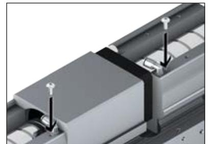
12. Wet the mounting holes for the roller carriages in the slide module with screw locking agent.
