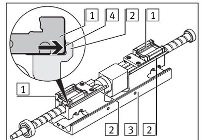
13. Wet the mounting holes in the roller carriages with screw locking agent.
