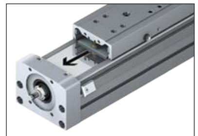
5. Unscrew the grub screws in the bearing block and bearing cap.
