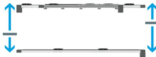
Lifts are added to the MCS<sup>®</sup> section and the transfer system combination. This is done for the return transport of the carriers below the process in the machine bed. This enables a compact system layout with unrestricted access from all sides, which is ideal for freestanding machines or production modules and standardised cell concepts.
