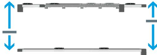
Lifts are added to the MCS<sup>®</sup> section and the transfer system combination. This is done to realise the return transport of the carriers below the process in the machine bed. This enables a compact system layout with unrestricted access from all sides, which is ideal for free-standing machines or production modules and standardised cell concepts.
