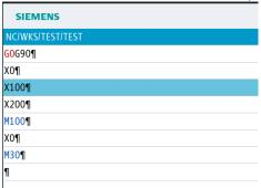
In this example, the NC program is paused at M-function "M100".
