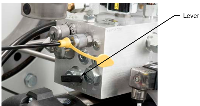
Figure 12. Depressurizing the hydraulic accumulator.
