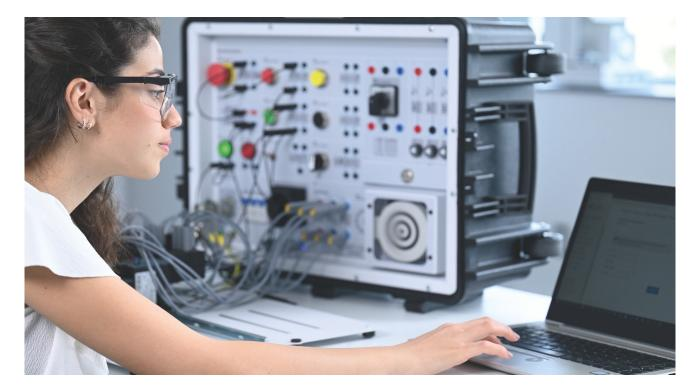
Students create control circuits by wiring power components (relays, contactors...) with a motor as well as control and protection devices. They learn to install, test, and troubleshoot the most common motor controllers through a varied range of learning activities.
