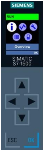
FIGURE 7.2-3 SPS MANUELL IN RUN
