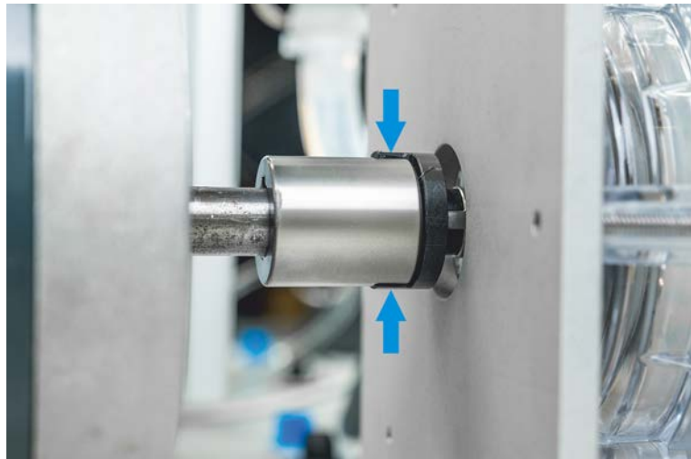
Figure 14: Compare how much the tang boot protrudes on each side of the coupling hub.
