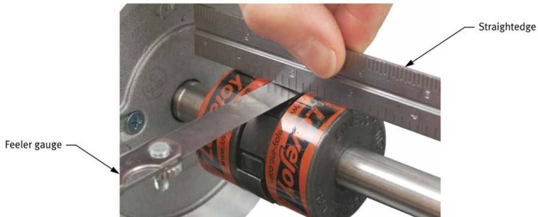
Figure 10: Straightedge and feeler gauge.
