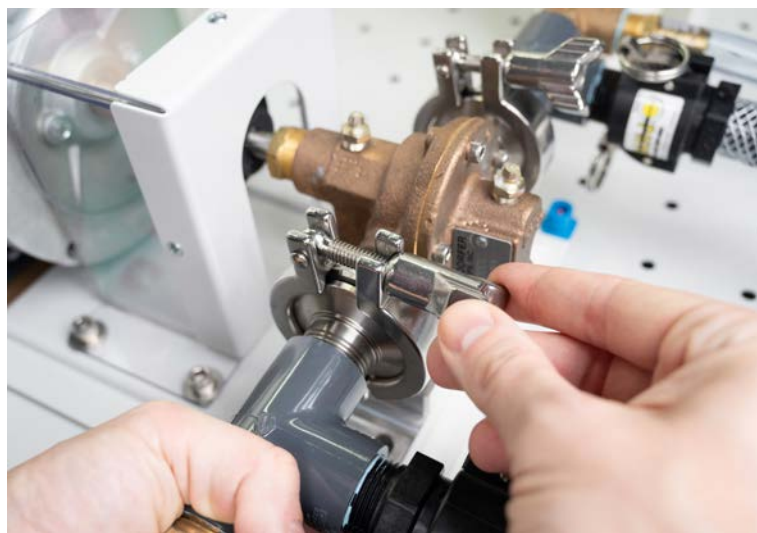
Figure 47: Locking the fittings using the wing nut.
