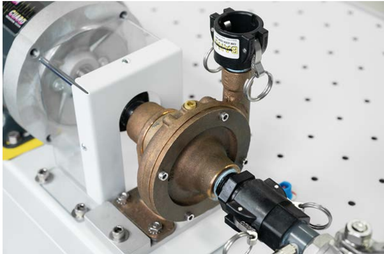
Figure 9: Brass plug used to prime the pump.
