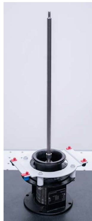
Figure 57: Pump with all stages removed.
