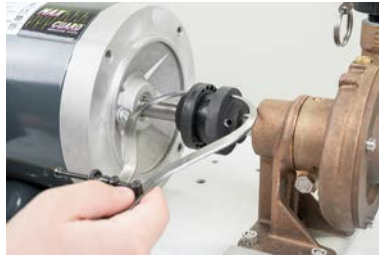
Figure 11: Angular misalignment measurement – Top.
