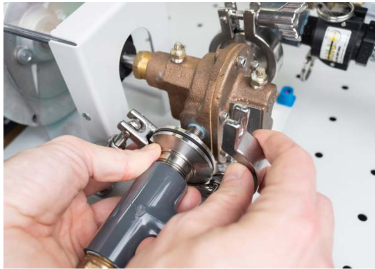
Figure 46: Placing the clamp on both fittings and closing the clamp.
