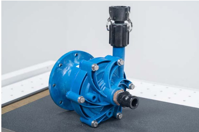
Figure 63: Magnetic drive centrifugal pump on the work surface.
