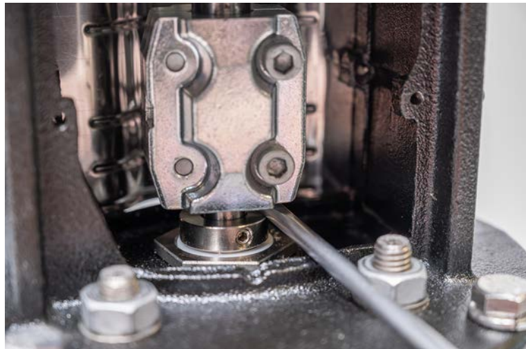
Figure 58: Lift the coupling so that the motor-shaft assembly does not drag on the motor stool.
