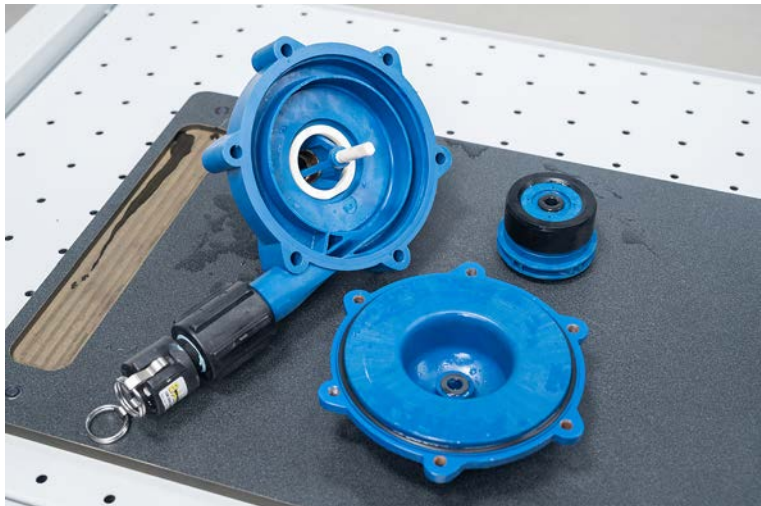
Figure 64: Inner components of the magnetic drive centrifugal pump.
