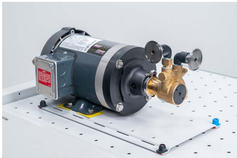
Figure 62: Vane pump attached to the motor.
