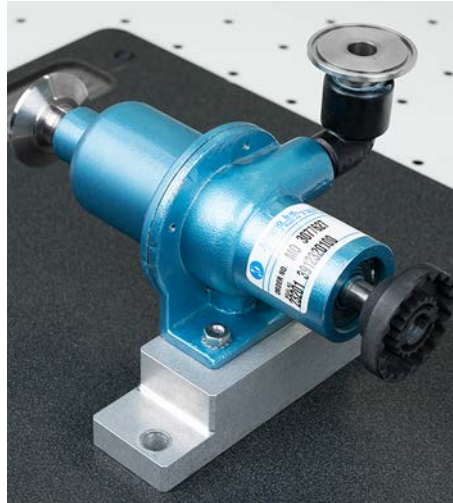
Figure 50: Progressive cavity pump on the work surface.
