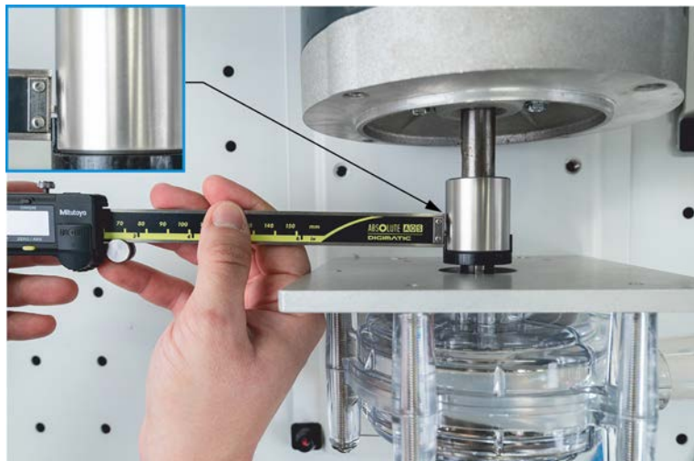
Figure 15: Measure the protrusion of the tang boot in vertical and horizontal positions (here with a digital caliper).
