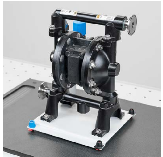
Figure 53: Pneumatic diaphragm pump on the work surface (back).
